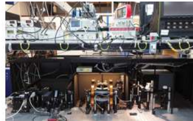
Equipment (right) to measure whether a protein found in the European robin's eyes is sensitive to the Earth's magnetic field
